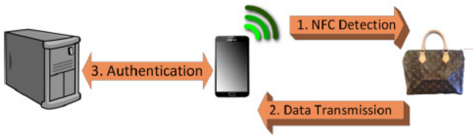
Figure 3.4-General flow of Anti-counterfeit Application
